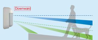
As the whole mirror units is adjustable vertically so that it is easy to fit to the slope ground. The upper stage zone should parallel the slope ground. The adjustable angle is  $\pm 5^{\circ}$  ( $\pm 1$ m at 12m away)
