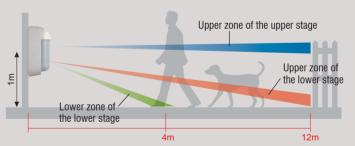
The lower stage sensor has 2 layer zones. In case masking the upper zone of the lower stage, the lower zone of the lower stage still cover the area near SIR05.
