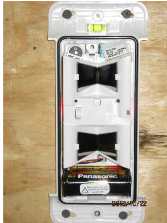
Photo 2: view of the inside of NVR780 PIR Detector
